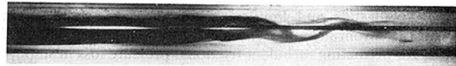
Fig. 5 Photograph of typical double helix dye pattern observed in the mockup of Walker's [34] geometry near a Reynolds number of 1560 ( Re^* = 1130 )
